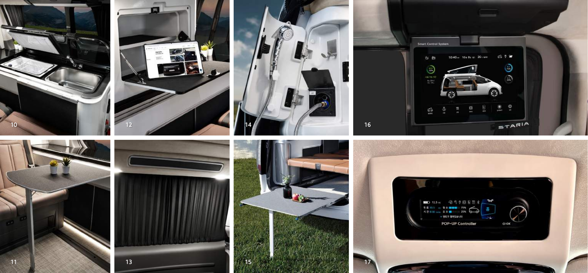
10. Sink Faucet Set & 36L Built-In Refrigerator 11. Folding Indoor Table _ Improved utilization of the indoor space. 12. 3rd Row Side Shelf _ The side shelf can also be used as a simple table. 13. BOSS speaker and rear curtain (Option) 14. Shower _ It is detachable, so you can take a simple outdoor shower. 15. Slide Rear Table _ It is fast and easy to install the outdoor table without tools. 16. 12.1-Inch Foldable Integrated Control Monitor (Controllable with Dedicated Application) _ Folding rotation method is applied. 17. Overhead Roof Controller _ You can conveniently operate POP-UP roof, lighting, heater, refrigerator/water pump/inverter functions from the first row.
