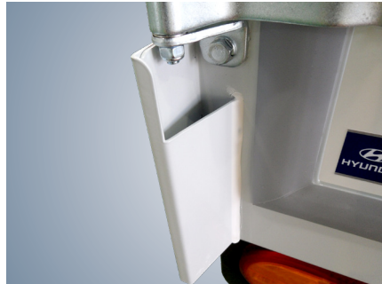
04 Rear Door Double Frame & Powder Coating
